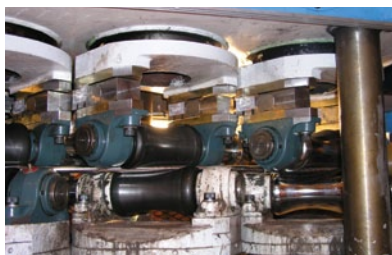
15. Roller straightening force system
