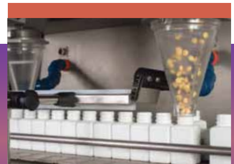
Strain-gage-based process weighing systems for batching and weighing in pharmaceutical production
